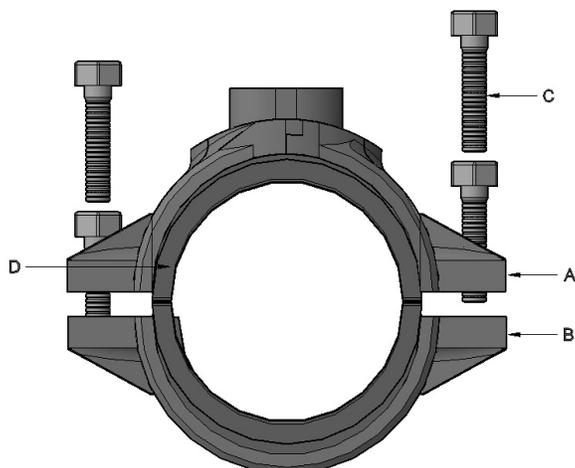
**MATERIAL:** HIERRO DUCTIL ASTM A-536
