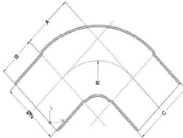
**MATERIAL: HIERRO DUCTIL ASTM A-536**
