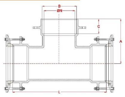
MATERIAL: HIERRO DUCTIL ASTM A-536 GRADO: 65-45-12
