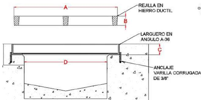
**MATERIAL REJILLA:** HIERRO DUCTIL ASTM A-536
